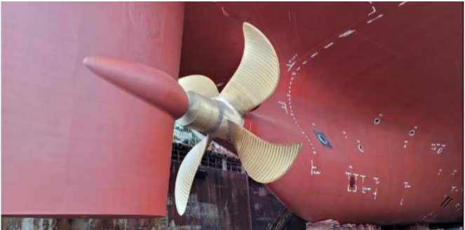
Propulsion Improving Device Installed on Newbuild Vessels (Rudder Bulb)
